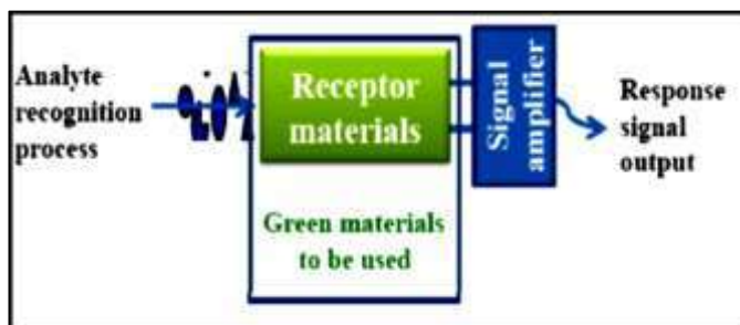
Fig. 4 Schematic representation of simplified working principle of a sensor
